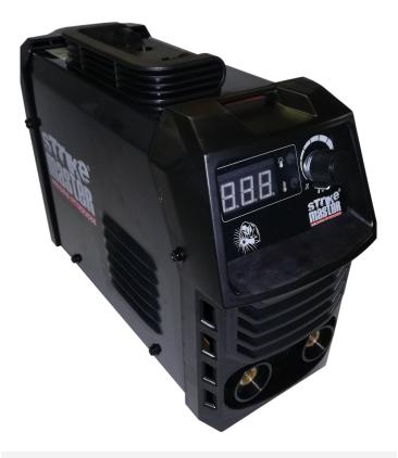
The Strikemaster MMA-161 is a 160A single phase, stick electrode welding machine which is designed on and manufactured to the latest digital inverter technology. It is compact, light weight with a single PCB allowing for easy mobility. The MMA-161 inverter machine ensures a clean, high quality weld and excels in basic and rutile electrode welding. Professional and DIY users can experience the built-in characteristics of anti-stick, hot-start and arc force.
