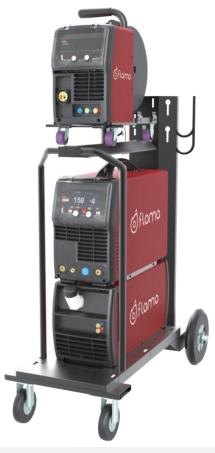
The Flama MIG 500F synergic is a 500A multi-purpose welding machine. Its inverter technology design is ideally suited for demanding industrial applications. The sturdy internal wire feeder can accommodate wire spools up to 20kg in weight. This robust machine has phase-loss protection, a high duty cycle, and a soft arc which ensures easy welding and produces high quality welds. This machine is ideally suited for the professional welder.
