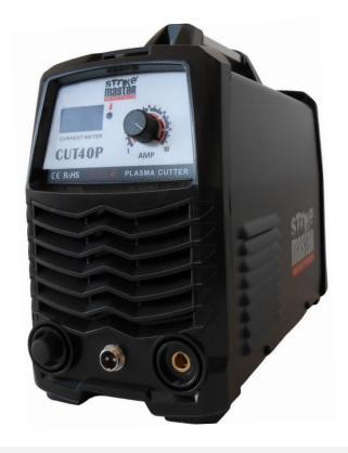
The Strikemaster CUT 40P is a new generation inverter plasma cutter designed on and manufactured to the latest IGBT technology and is characterised by its performance and high efficiency. It delivers clean and straight cuts at adjustable currents up to 40A. It is equipped with a pilot ignition, is reliable, light-weight and easy to use. Conductive materials such as standard steel, stainless steel, aluminium, brass, copper and titanium can be cut hassle free.
