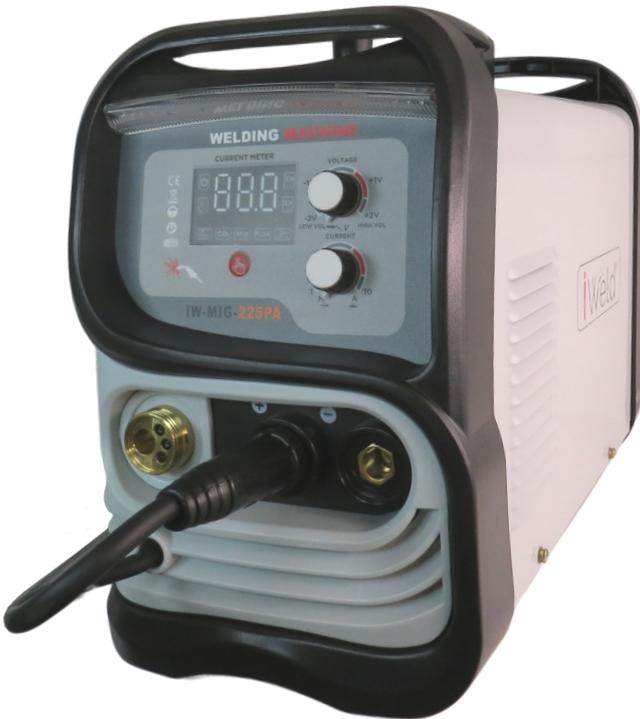
The iWeld MIG-225PA SYNERGIC is a 225A single phase, 220V MIG multi-purpose welding machine which is designed on and manufactured to the latest digital inverter technology. It supports MIG, MAG, LIFT TIG and MMA welding processes. The machine is extremely portable and can accommodate a wire spool of up to 5 kg. It is ideal for on-site work due to its light mass and diverse applications. Its characteristics ideally suit professionals and DIY users.
