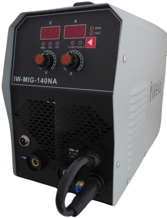
The iWeld MIG-140NA is a 140A single phase, 220V MIG multi-purpose welding machine which is designed on and manufactured to the latest digital inverter technology. It supports MIG, LIFT TIG and MMA welding processes. The machine is extremely portable and can accommodate a wire spool of up to 5 kg. It is ideal for on-site work due to its light mass and diverse applications. Its characteristics ideally suit professionals and DIY users.
