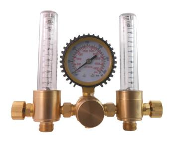
The TAURUS FLOWMETER DOUBLE OUTLET ARGON TARG1-DOFM connects to an argon gas cylinder. It's a single cylinder inlet with a dual outlet flowmeter. Its function is to individually adjust each outlet and measure the amount of gas passing through separately. It is generally used in TIG and MIG welding. The adjustment knob adjusts the flowrate and not the pressure. The flowrate is set in litres per minute. The gauge measures the inlet pressure and each tube measures the delivery flowrate.
