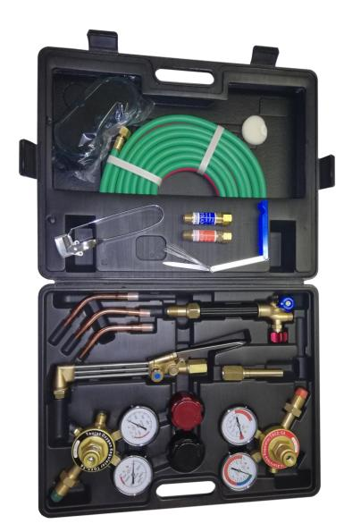
The TAURUS combination kit is a starting kit for general brazing, welding and cutting with oxygen and acetylene gas. It can be extended to suit personal and job requirements. The equipment is presented in a secure, robust toolbox. The inlet fittings on the regulators are G 5/8" - B-rh on the oxygen side and B-lh on the acetylene side. The fittings are compatible with industrial size gas cylinders in South Africa.
