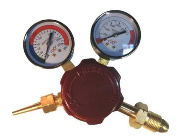
The primary function of a gas regulator is to reduce high-pressure gas in a cylinder or process line to a lower, more usable level. A regulator is not a flow control device. It is used to control delivery pressure only. It has two gauges, one to measure the inlet pressure and the other to measure the outlet delivery pressure.
