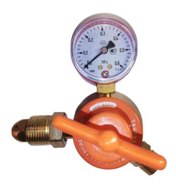
The primary function of a gas regulator is to reduce high-pressure gas in a cylinder or process line to a lower, more usable level. A regulator is not a flow control device. It is used to control delivery pressure only.
