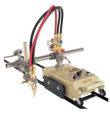
The straight line cutter CG1-30 is a light, portable machine running on rails which can be extended to suit the cutting length. It uses oxygen-acetylene or oxygen-LPG. The traveling speed is adjustable enabling cutting through materials up to 100mm thick. Cutting nozzles ANME/ANM and PNME/PNM used on the universal cutting torch, can both be fitted to the machine.
